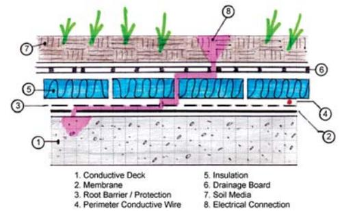
Figure 4 - ELD section with overburden in place.
