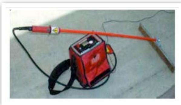
A continuous higher voltage charge than produced by the low voltage pulse generator is delivered from the generator to the piece of testing equipment. With the electrical potential difference between the grounded roof deck and high voltage testing equipment we essentially have two electric plates. If there are any breaches or punctures through the waterproofing membrane, which acts as an electric insulator, the electric current will ground itself at the breach.
